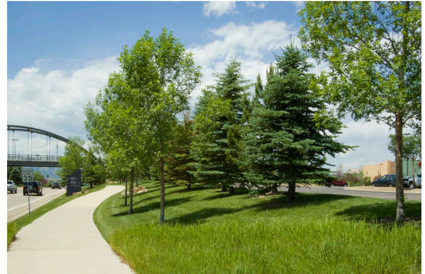
Figure 4.c: This planted berm is a good buffer from the highway.
